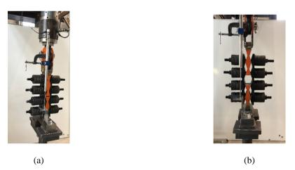
Figure 9. RSFJ component testing: (a) setup, (b) RSFJ at the maximum designed displacement (60 mm)
